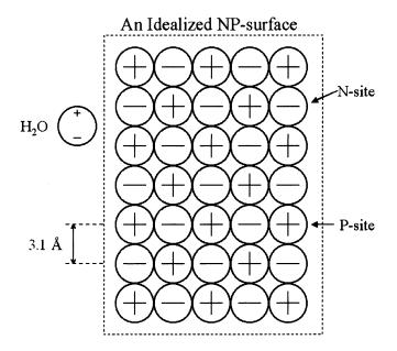
FIGURE 7. An Idealized NP surface. The distance between a pair of the nearest-neighboring N and P site is equal to the distance, r, between neighboring water molecules in the normal liquid state and equal to 3.1 Å.(From Ling 2003)
