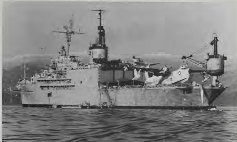
The seaplane tender *Salisbury Sound* (AV-13) supporting SP-5B flying boats at Cam Ranh Bay. Note the SP-5B resting on her fantail, hoisted aboard by the 30-ton-capacity cranes on the fantail and atop the ship's amidships hangar. These tenders were large ships, displacing over 15,000 tons full load, and manned by a crew of about one thousand. (U.S. Navy, R.D. Moeser)
