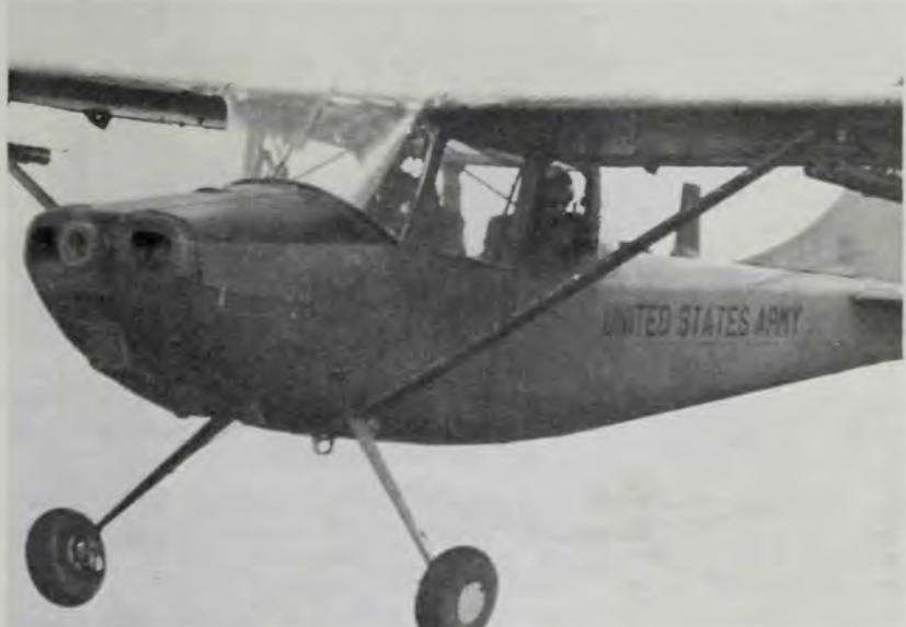
The Marine Corps' own O-1E Bird Dogs reached the end of their service lives and the Marines had to quickly borrow additional aircraft from the Army, without having time to repaint the two-seat Cessnas in Marine markings. Taken in 1968, this photograph shows two Marine crewmen on a low level photo reconnaissance flight in an O-1E still bearing Army identification. Note the smoke rocket canisters under the wing. (U.S. Marine Corps)
