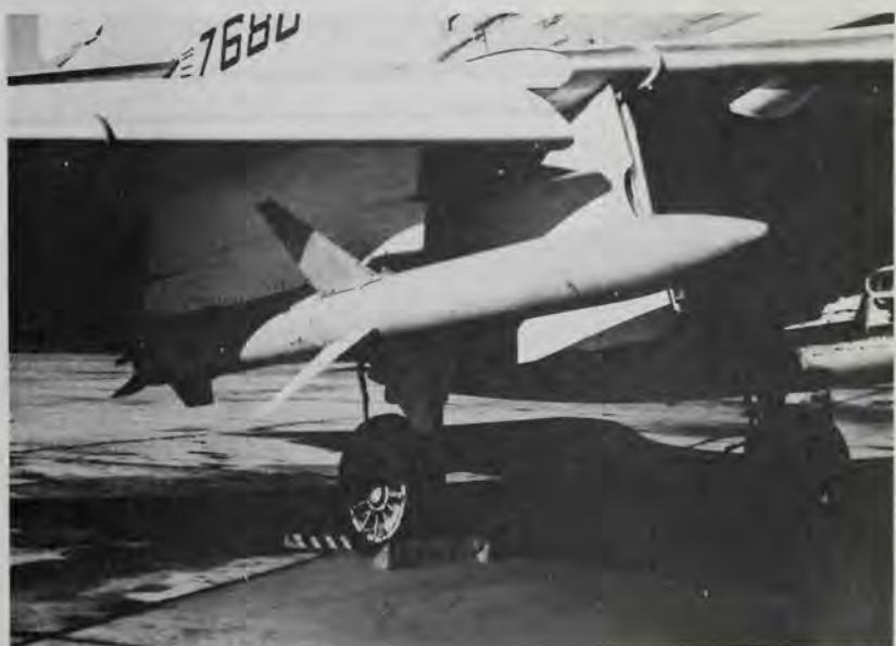
The innocuous-looking AGM-45A Shrike, mounted here on an A-4C Skyhawk, was used by the Navy and Air Force in Vietnam from 1966 onward. An anti-radiation missile (ARM), Shrike was intended to "home" on enemy antiaircraft radars. Countermeasures were developed, and then counter-countermeasures in the see-saw electronic phases of the Vietnam conflict. (U.S. Navy, F.W. Pickrell)
