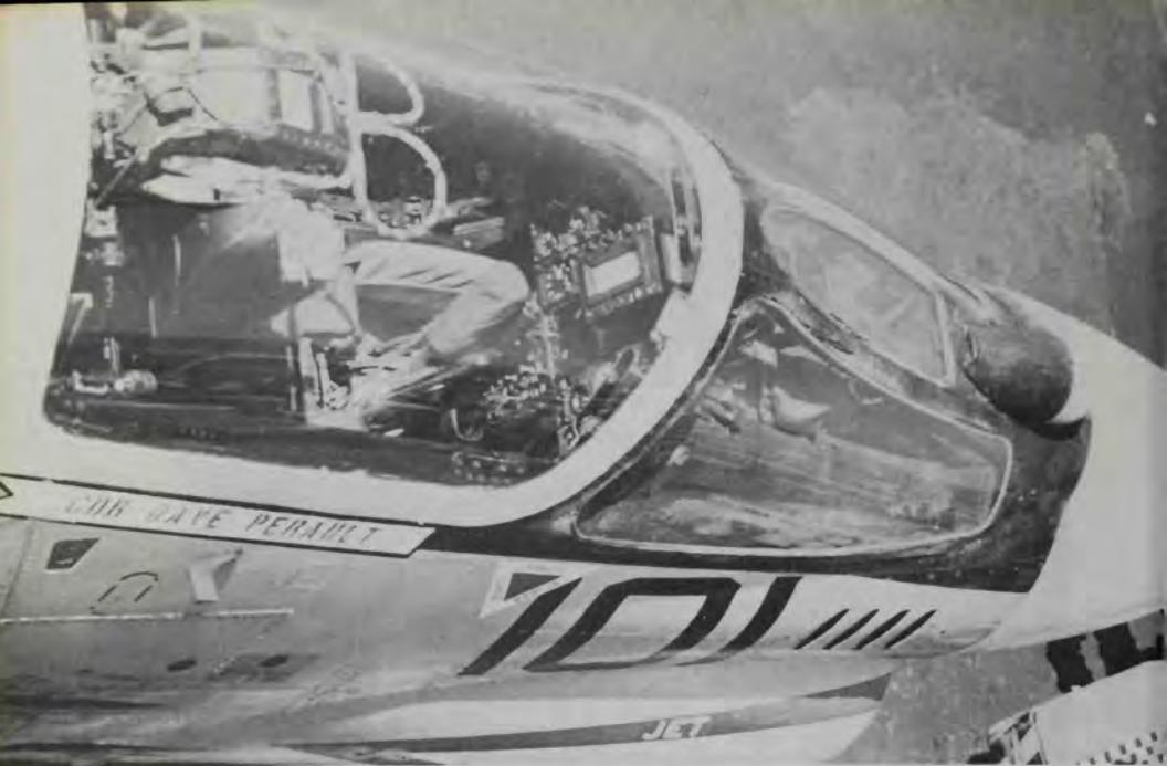
The Hot Seat. The cockpit of an F-8 Crusader is small, cramped, and complex. This aircraft was flown by Commander Dave Perault, commanding officer of VF-24 aboard the *Hancock*. The two rings above the seat are handles to activate the ejection seat; the white rectangle forward of the seat is the radar screen. (Eliot Tozer)
