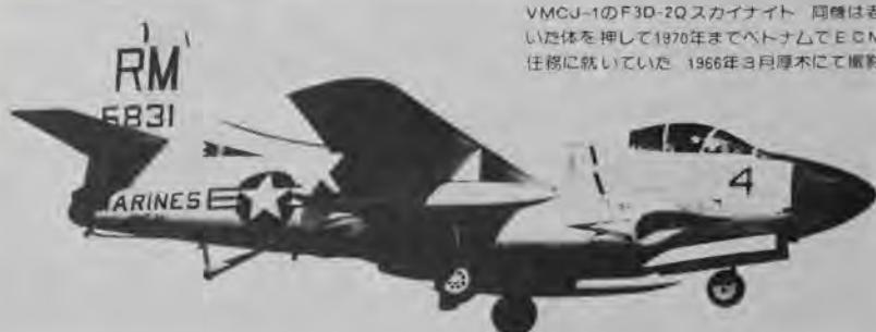
An EF-10B Skyknight (formerly F3D-2Q) from Marine Composite Reconnaissance Squadron (VMCJ) 1 was one of the oldest aircraft used in combat in Vietnam. The Skyknights, modified from night fighters, were used for electronic surveillance and intelligence.
