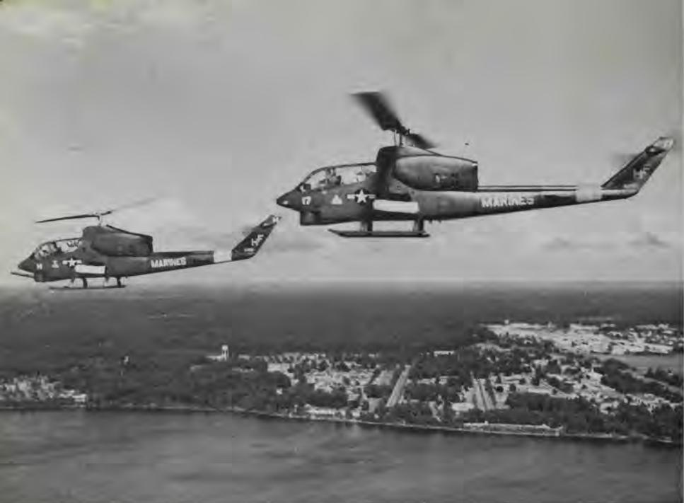
The Bell AH-1J SeaCobra, designed specifically for the Marine Corps, was ordered into production in May 1968. Although the Cobra's fuselage was radically different than that of the basic "Huey," the AH-1G had the earlier helicopter's engine, transmission, and rotor system. A three-barrel 20-mm gun is mounted in the chin turret and rocket pods are carried on the stub wings. (U.S. Marine Corps, S. Powell)
