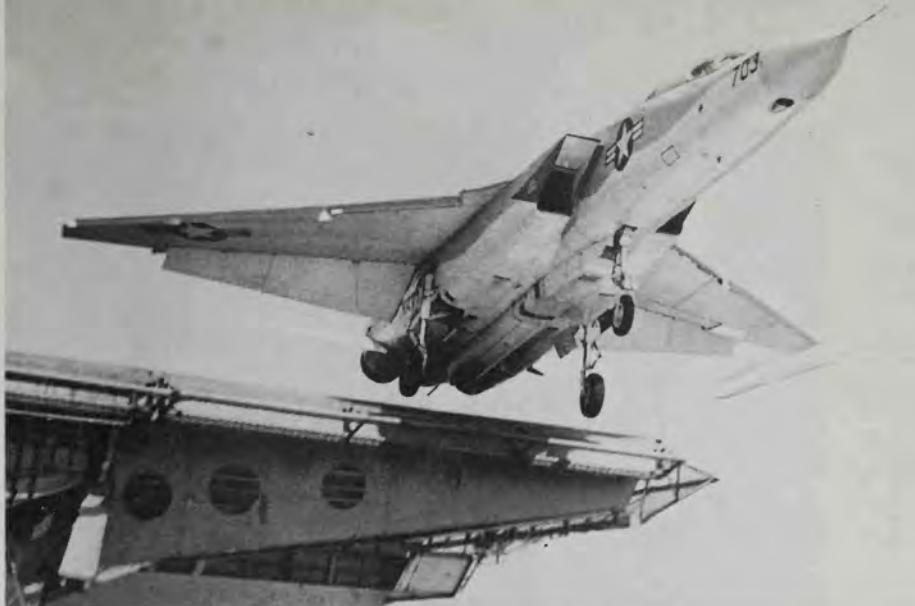
An RA-5C "Viggle" is catapulted from the carrier *Ranger* for a reconnaissance mission over North Vietnam. Developed from the A-5 (A3J) supersonic strike aircraft, the RA-5C variant carried five camera systems plus Side-Looking Aircraft Radar (SLAR) and Electronic Countermeasures (ECM) equipment. Weapons could still be carried internally or on wing pylons, but the aircraft were employed in Vietnam only in the recce role. (U.S. Navy, Donald Granthan)
