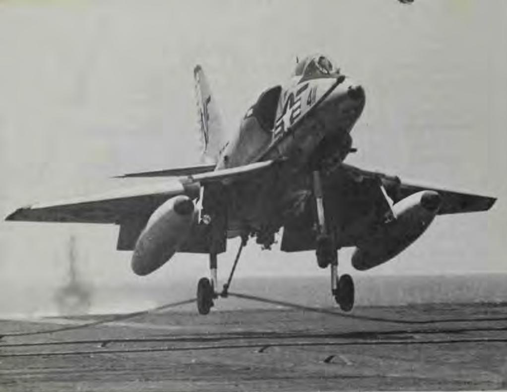
This A-4 Skyhawk has just caught the No. 1 wire while coming aboard the carrier *Hancock* after a mission over North Vietnam. Barely visible under the aircraft's right wing is the plane guard destroyer, steaming in the carrier's wake to pick up the crew of any aircraft that "goes into the drink" during flight operations. (U.S. Navy, R.D. Moeser)
