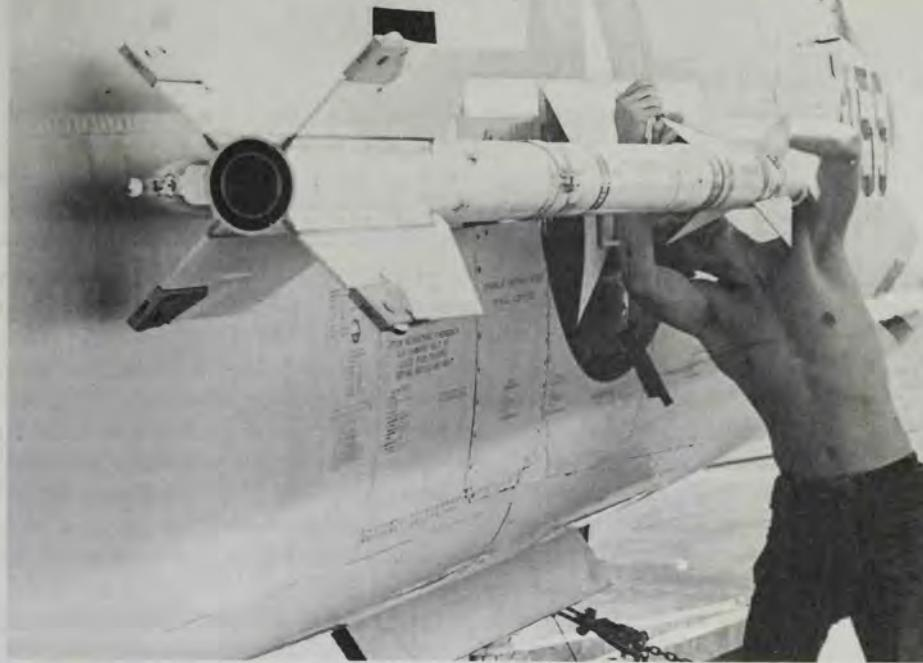
An aviation ordnanceman attaches a Sidewinder heat-seeking, air-to-air missile to an F-8 Crusader aboard the *Bon Homme Richard*. The Crusader was the principal U.S. naval fighter during the early Vietnam War, carrying missiles and bombs in addition to an internal gun armament. The F-4B Phantom, which replaced the Crusader aboard larger carriers, did not have a gun armament. (U.S. Navy, R.D. Moeser)
