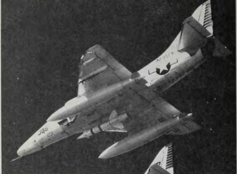
An A-4E Skyhawk of VA-72 in flight with two drop tanks and an AGM-12 Bullpup-A missile on its centerline pylon. The A model carried a 250-pound bomb as warhead and could be released up to seven miles from the target; the Bullpup-B carried a 1,000-pound bomb with slightly more range. An A-4 would carry up to three Bullpups. The missiles required the plane to continue to fly straight after launch to help guide the missile. (U.S. Navy)
