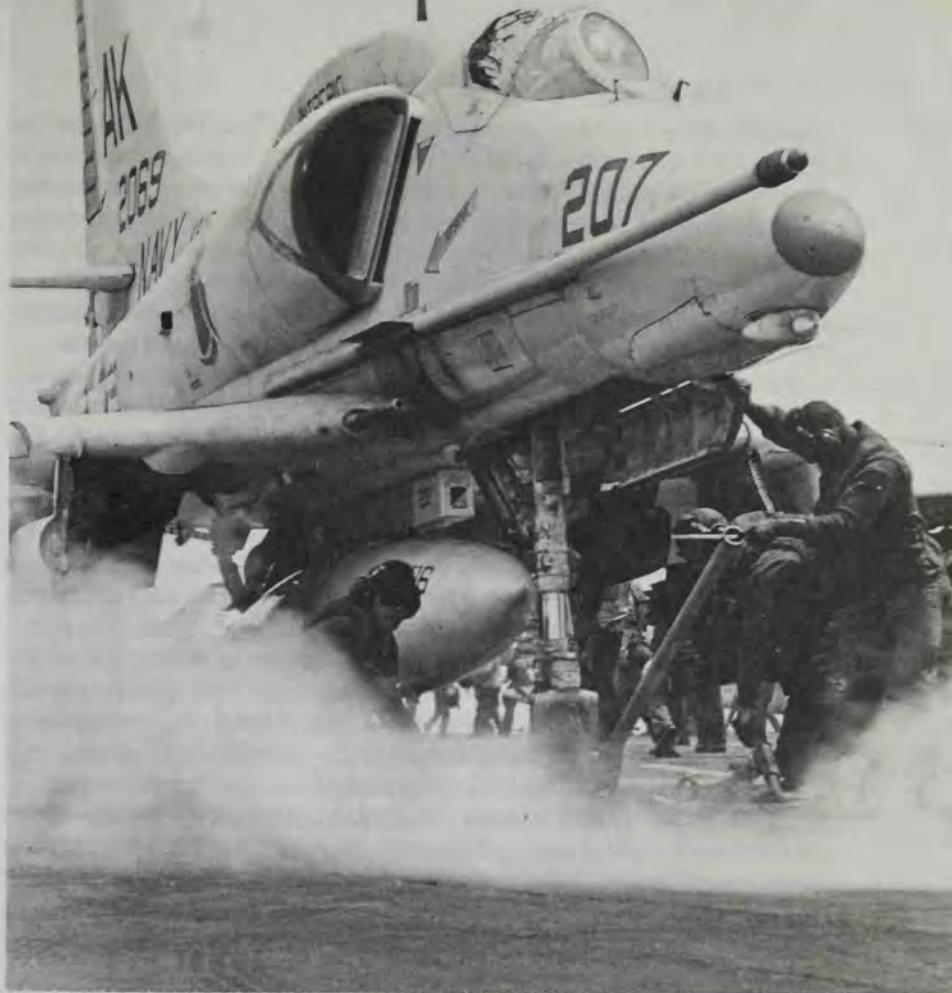
An A-4F Skyhawk is readied on a catapult aboard the carrier *Intrepid* in the Gulf of Tonkin. The flight-deck crewman at right is adjusting the A-4F on the catapult with a steering bar. The plane has a centerline drop tank and bombs on its wing pylons. Note the 20-mm cannon in the wing root and the refueling probe. (U.S. Navy, John G. Jacob)
