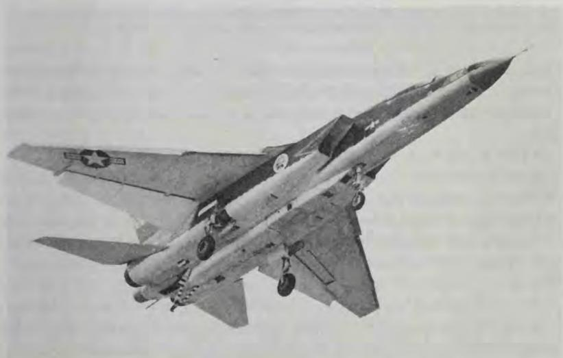
A "Vigie" with hook and wheels down, and flaps extended, roars in for a landing aboard a carrier. The openings for cameras in the sensor pod are visible just behind the nosewheel. (U.S. Navy)
