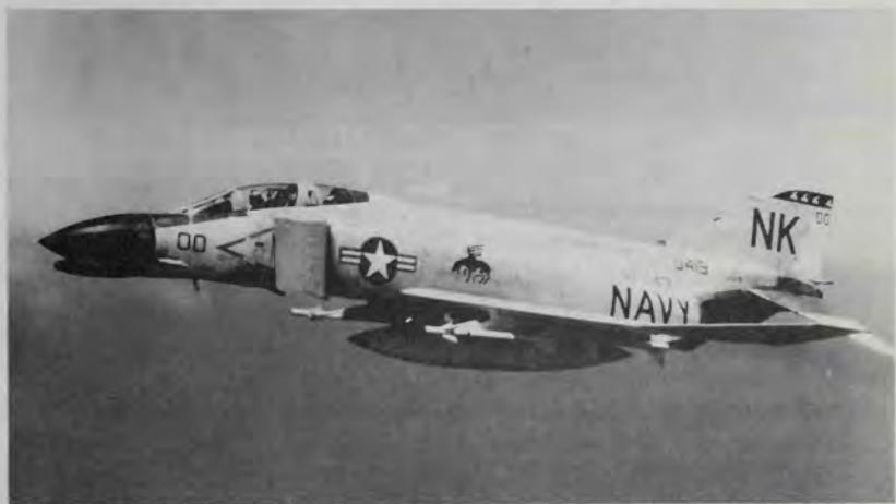
The Phantom was unquestionably the best fighter aircraft of the 1960s. This F-4B variant, armed with Sidewinder air-to-air missiles, is from VF-143 aboard the *Constellation*. The "00" or "double nut" marking indicates that it is flown by the air wing commander—always called "CAG" for air group commander despite the redesignation as carrier wings in 1962. (U.S. Navy)
