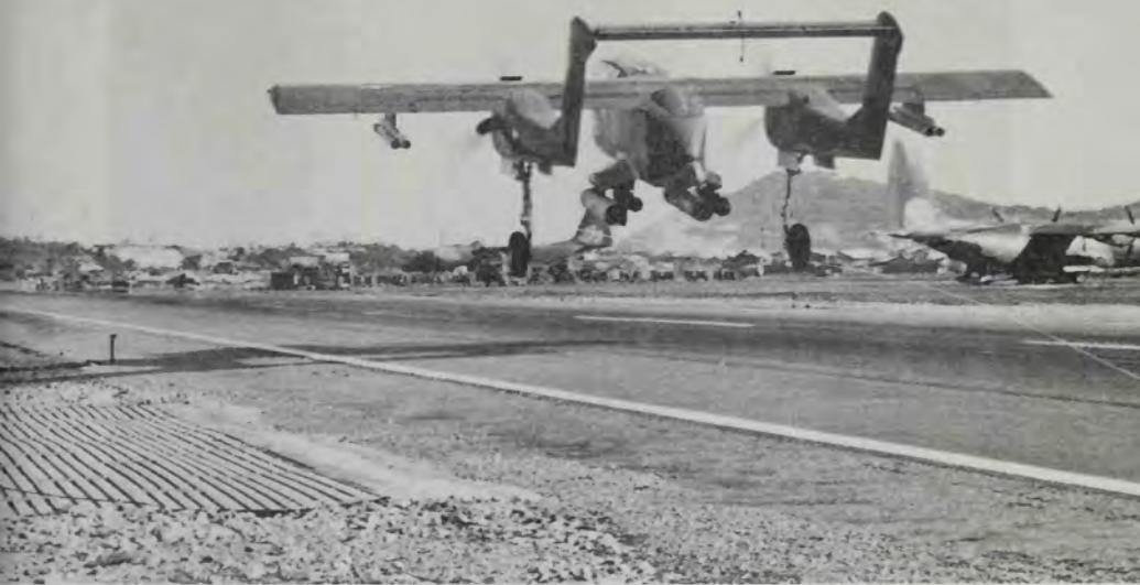
A rocket-armed OV-10A Bronco takes off from Vung Tau in South Vietnam. The OV-10A is a STOL (Short Take-Off and Landing) aircraft, and subsequently the planes have operated from helicopter carriers without the use of catapults or arresting gear. (U.S. Navy, A.R. Hill)
