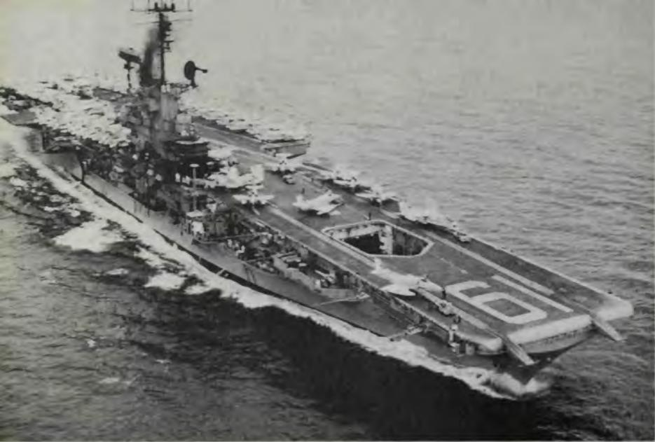
The *Hancock*, one of the extensively modernized Essex-class (CV-9) carriers, was the smallest type of flattop to operate in the Vietnam War. Their air wings were limited in that they could not operate the larger F-4 Phantoms and A-6 Intruders when those aircraft became available. During a lull in flight operations the *Hancock*'s forward elevator is in the lowered position. (U.S. Navy, L.P. Bodine)
