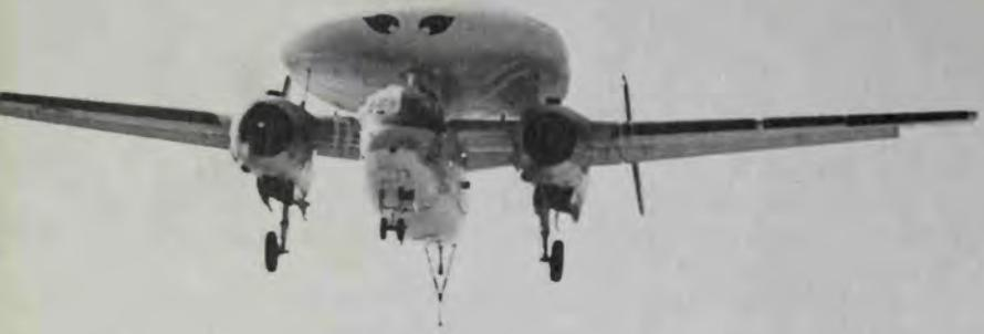
An E-1B Tracer early-warning aircraft comes in to land aboard the carrier *Hancock* during operations off Vietnam. The saucer atop the plane houses a rotating AN/APS-82 radar antenna. (Eliot Tozer)
