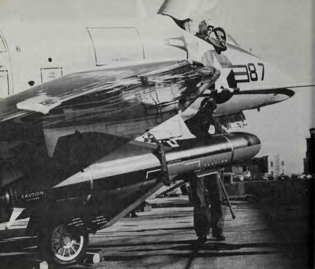
The AGM-62 Walleye glide bomb was the most accurate and effective air-to-surface weapon of its time, despite being unpowered. It was fitted with a self-homing television guidance system that controlled direction by moving control surfaces on the stub wings. The "missile," which carried an 850-pound warhead, is shown here during tests with an A-4 Skyhawk. (U.S. Navy)
