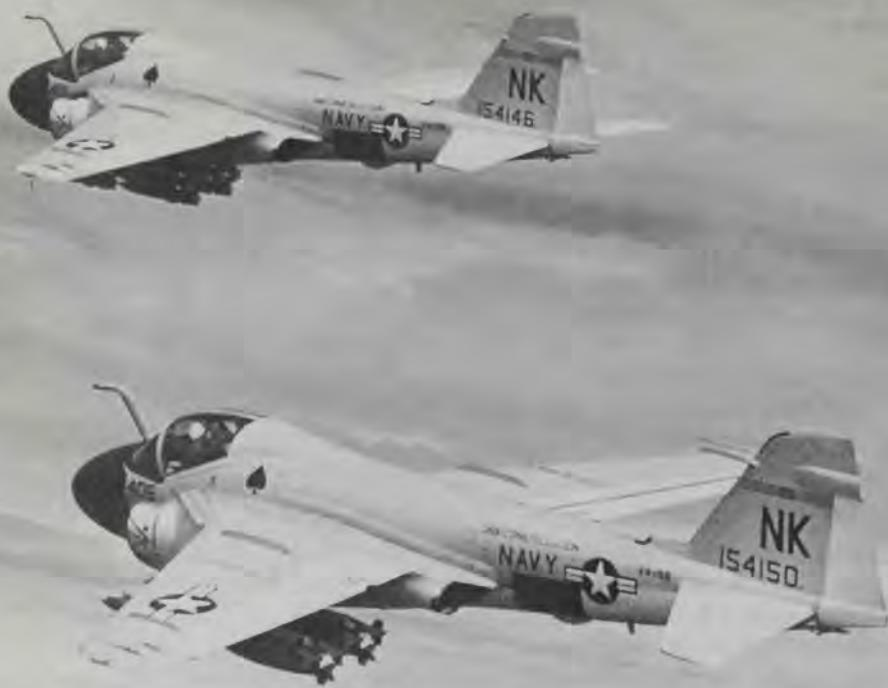
A-6A Intruders from the carrier *Constellation* set off on a bombing mission. These VA-156 aircraft show the Intruder's awkward appearance: thick forward fuselage with side-by-side seating for the pilot and, slightly behind him to his right, the bombardier/navigator; the narrow tail; and the refueling probe projecting up just forward of the cockpit. (U.S. Navy)
