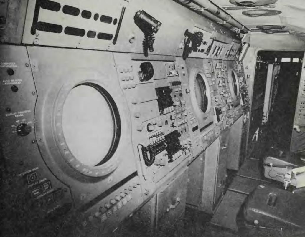
The fuselage of the E-2 Hawkeye is crammed with electronic equipment plus displays for three operators. The cockpits, for pilot and copilot, are beyond the doorway at right. In the Airborne Early Warning (AEW) role the Hawkeye can detect hostile aircraft and direct friendly fighter or attack planes. (Grumman)
