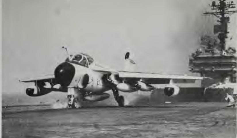
A prototype EA-6A Prowler electronic warfare aircraft being catapulted from a *Forrestal*-class carrier is loaded with four electronic jamming pods plus three drop tanks. The Marine Corps took delivery of all twenty-one EA-6A variants of the Intruder, with the Navy flying only the more capable EA-6B model. (U.S. Navy)
