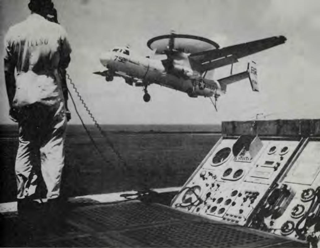
An E-2A Hawkeye lands aboard the carrier *Constellation* in the South China Sea. In the foreground the landing signal officer (LSO) uses instruments and a telephone in place of the twin paddles used by his predecessors in World War II. Note the aircraft's large turboprop engines, four-fin tail, and distinctive rotating radome. (U.S. Navy, Robert K. Drudge)
