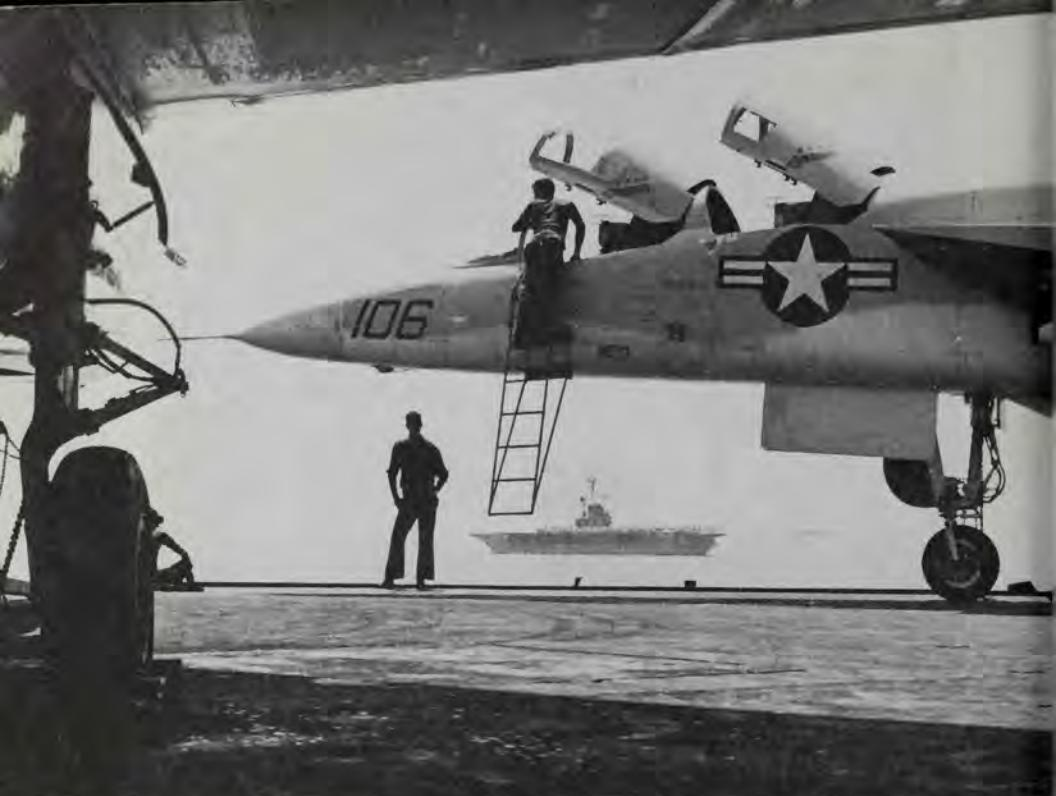
An RA-5C is checked out aboard the carrier *Ranger* in the South China Sea. The smaller *Hancock* and a destroyer steam nearby. Note the tandem seating arrangement for the pilot and reconnaissance systems operator. The sleek RA-5C was rated at speeds of Mach 1 at sea level and Mach 2 at about 40,000 feet. In the strike configuration a nuclear weapon could be carried internally as well as on four wing pylons. (U.S. Navy, Jean Cote and R.D. Moeser)
