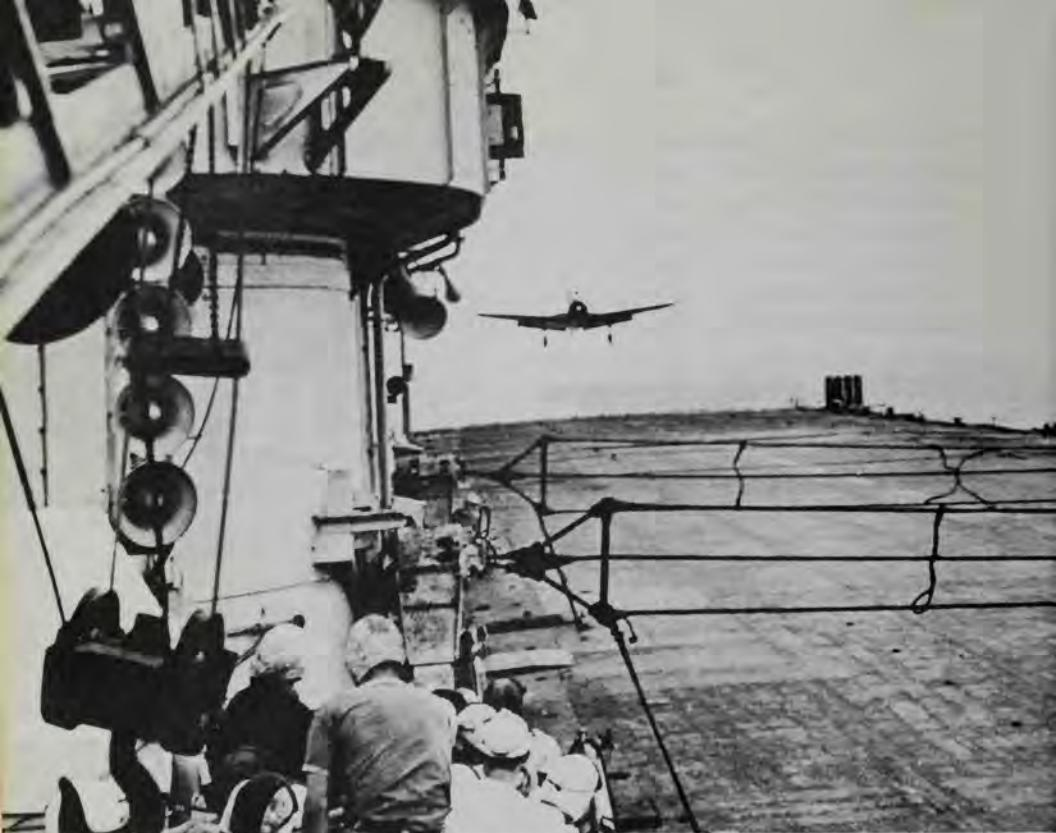
An SB2C Helldiver comes in for a landing aboard the French carrier *Arromanches*. In the foreground are wire barriers, to halt the aircraft should it miss the arresting wires. Before the development of angled or canted flight decks, a plane that missed the arresting wires would crash into planes forward if not halted by the barrier. (French Navy)
