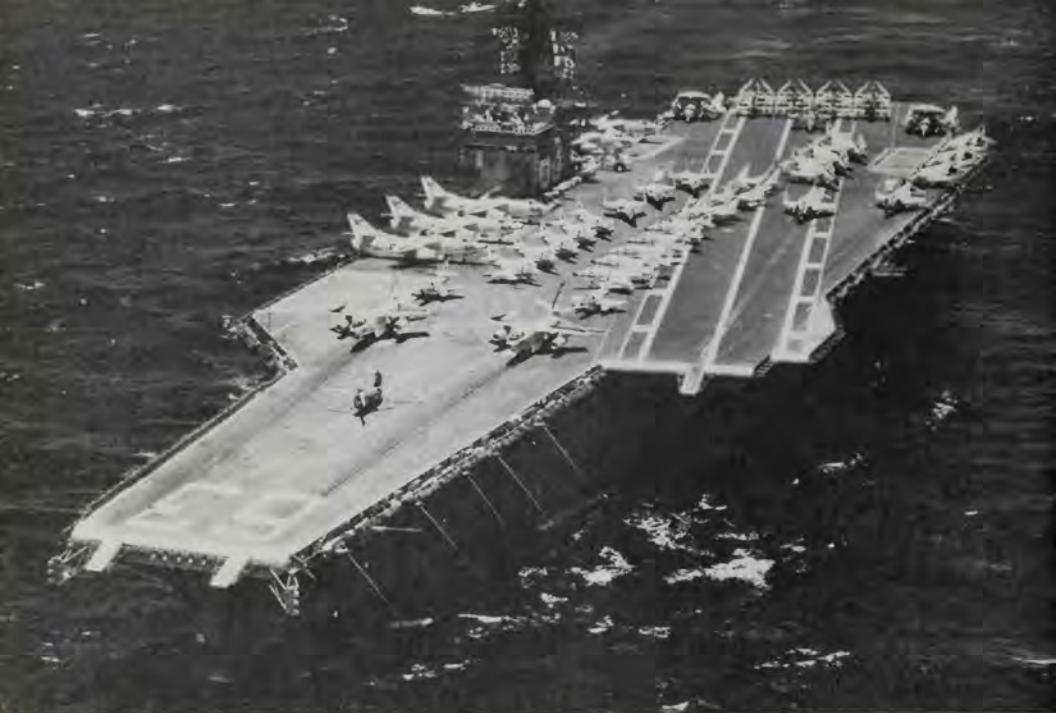
The *Kitty Hawk* at sea. One of the *Forrestal*-class "super" carriers, she can operate up to ninety aircraft. In this photo a pair of 35-ton A-3B Skywarriors sit on her forward catapults, and a pair of F-4B Phantom fighters are on the two angled-deck catapults. Note the markings of the angled deck, which permit a plane missing an arresting wire to accelerate and take off for another landing run. (U.S. Navy)
