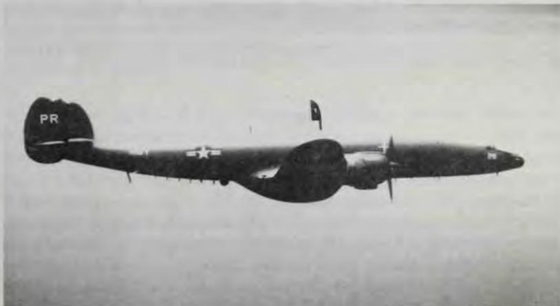
A Navy-flown EC-121 Warning Star similar to this aircraft was shot down over international waters in April 1969 by the North Koreans. The large, land-based military version of the Lockheed Constellation was used for electronic surveillance, with the ventral and belly domes housing AN/APS-20 and -45 search radars. (U.S. Navy)
