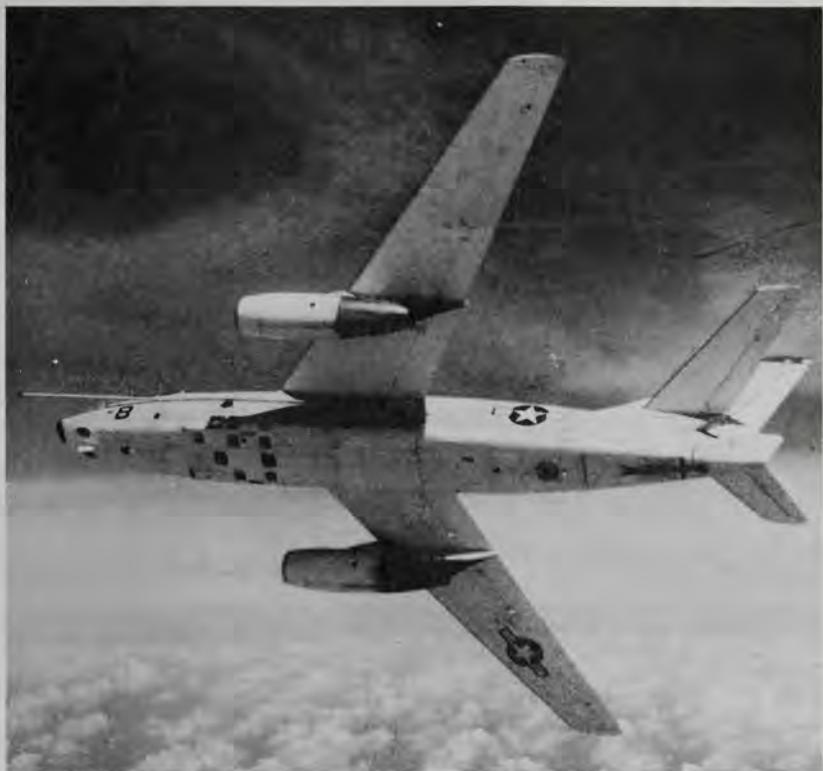
An RA-3B Skywarrior shows off its camera lens. This version of the venerable "Whale" had twelve camera stations plus stowage for extra film, and an arsenal of flash bombs for night photography. The plane was flown by a crew of three: pilot, photo-navigator-assistant pilot, and photo technician. Note the carrier arresting hook retracted into the tail. (U.S. Navy, C. Larson)
