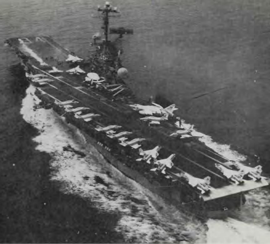
An A-4F Skyhawk goes off the No. 2 catapult of the *Oriskany* during a launch in the South China Sea. The dark rectangle on the starboard side aft of the "island" is the deck-edge elevator swung to a vertical position, indicating that the ship recently has or will soon refuel from a fleet oiler. An EKA-3A Skywarrior parked next to the elevator dominates the flight deck. (U.S. Navy, R.A. Long)
