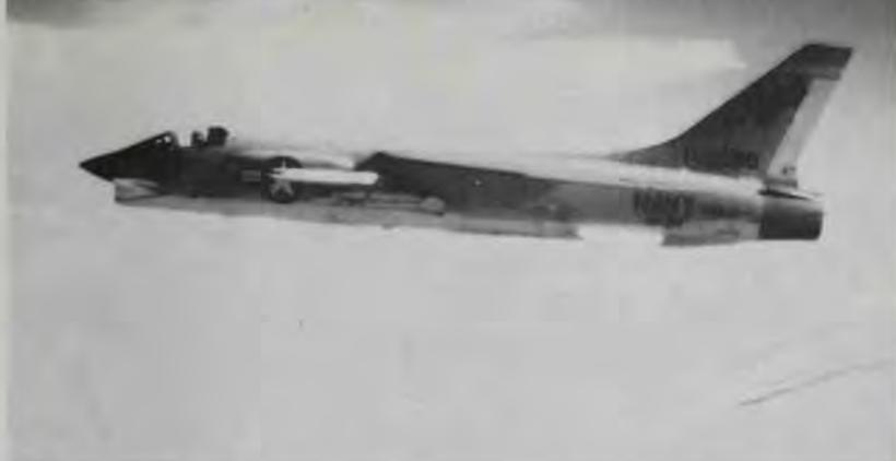
An F-8 Crusader from VF-24 aboard the *Hancock* shows the aircraft's clean lines and the location of air-to-air missiles, in this view Sidewinder missiles and Zuni rockets, on "cheek" attachment points just behind the national insignia. This F-8 is from Fighter Squadron (VF) 24 of Carrier Air Wing (CVW) 21, indicated by the tail letters "NP." Most Atlantic Fleet air wings have an identification code beginning with "A" and Pacific Fleet wings with "N." (Courtesy Tom Irwin)
