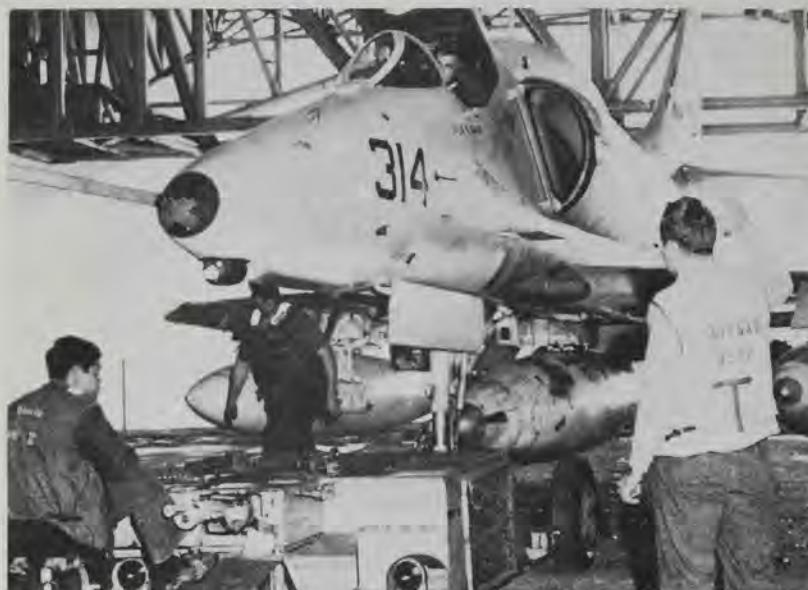
Getting ready: an A-4F Skyhawk from VA-212 receives tender loving care from hangar deck personnel aboard the *Hancock*. Two drop tanks and a center-line in-flight refueling pod is fitted to this plane, to permit it to refuel other A-4s in flight.
