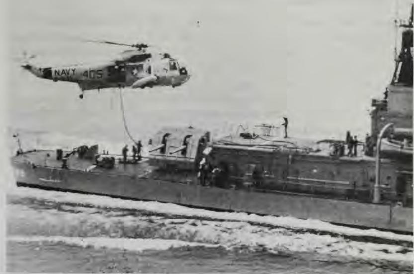
An SH-3A Sea King helicopter from Helicopter Antisubmarine Squadron (HS) 84 refuels while hovering over the destroyer *Henderson* (DD-785). This technique enabled search and rescue helicopters to remain aloft over the Tonkin Gulf during carrier operations, especially when the helicopters were kept immediately offshore to rescue downed pilots. The helicopters could land on the larger cruisers to rest and refuel. The destroyer flight decks could not handle the Sea Kings. (U.S. Navy, E.P. Carr)
