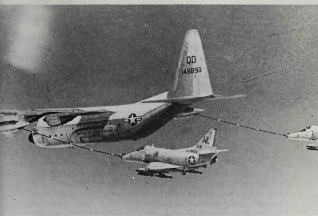
A pair of Marine A-4 Skyhawks are refueled in flight some 10,000 feet above South Vietnam by a KC-130 Hercules. Marine "Herks" from Refueler/Transport Squadron (VMGR) 152 provided air-to-air fueling of tactical aircraft as well as cargo and troop transport services in Vietnam. Refueling permitted the Skyhawks to take off with large bomb loads and minimum fuel. (U.S. Marine Corps, Carl E. Erickson)
