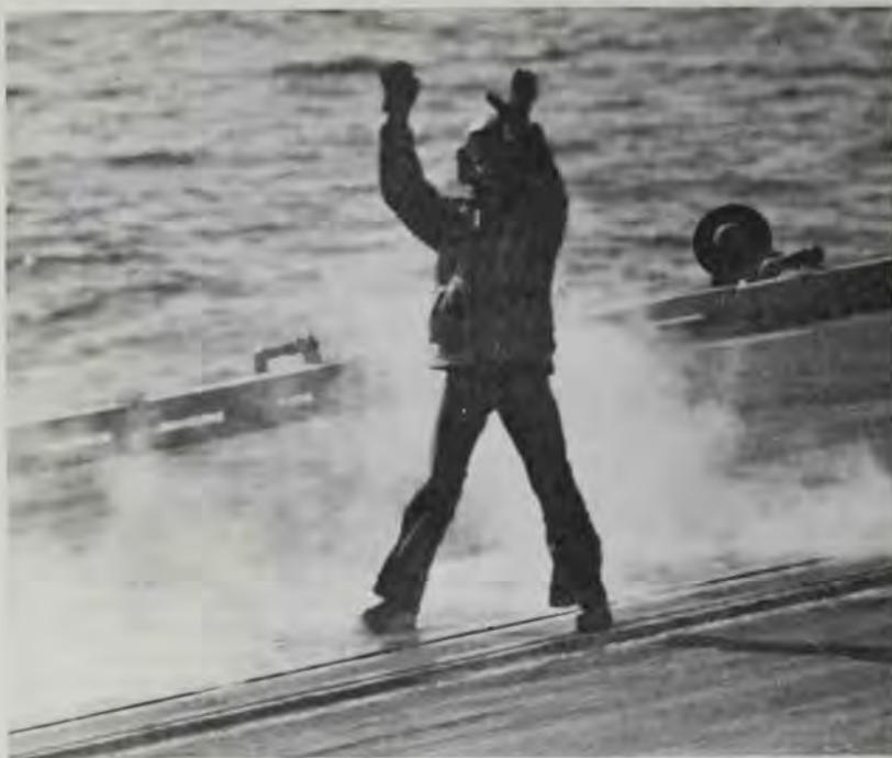
A flight deck director guides a plane onto a steam catapult in preparation for a launch, as the carrier steams in the Gulf of Tonkin. The officer is straddling the catapult track, from which wisps of steam are escaping. (U.S. Navy)
