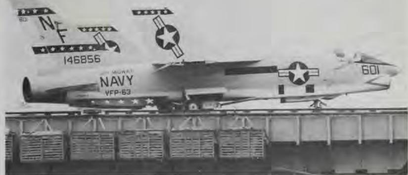
During the final days of South Vietnam and in the *Mayaguez* crisis, reconnaissance aircraft again had an important role. This RF-8G Photo Crusader from VFP-63 aboard the *Midway* was rebuilt from an RF-8A. Note the relatively small area of the wings that fold for carrier stowage. (Hideki Nagakubo)
