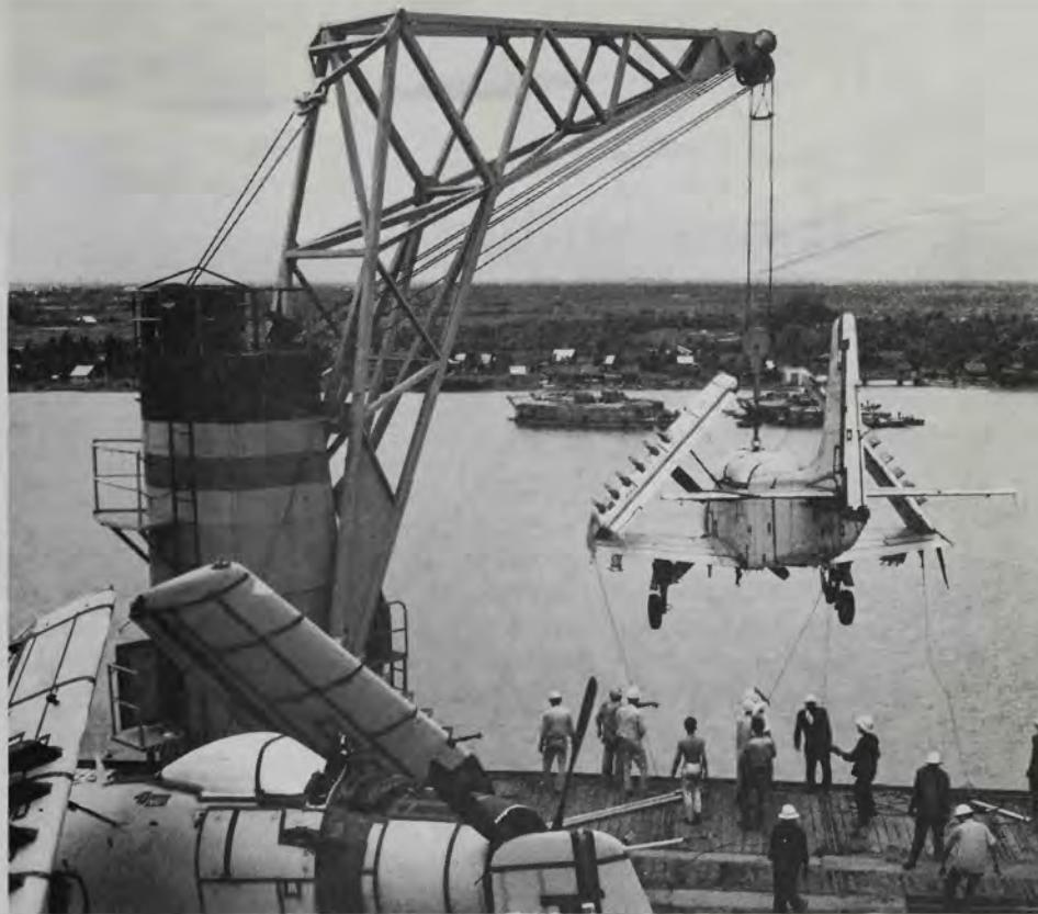
An A-1 Skyraider is lifted off the *Core* and lowered onto a waiting barge. The former jeep carrier transported seventy aircraft on this particular transit. The MSTS ships were civilian-manned by Civil Service crews. Note the preservative materials covering the Skyraiders to protect them from salt and spray during the Pacific crossing. (U.S. Navy)
