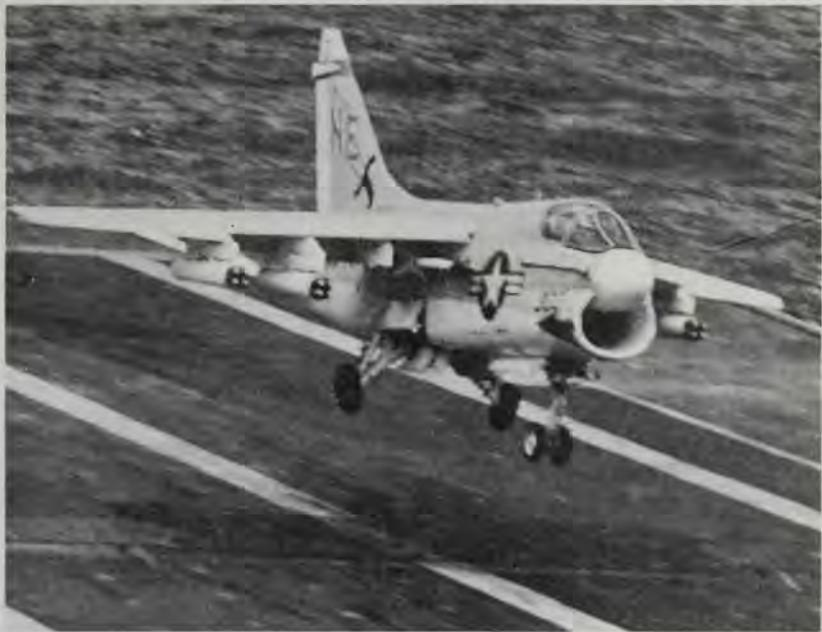
An A-7A Corsair lands aboard the carrier *Ranger* in the Gulf of Tonkin after a mission over North Vietnam. The VA-147 aircraft still has four rocket pods on its wing pylons, plus Sidewinder air-to-air missiles on its "cheek" attachment points. Note the superficial resemblance to the F-8 Crusader. The A-7's cockpit is closer to the nose and the wing does not move upward as in the fighter. (U.S. Navy)
