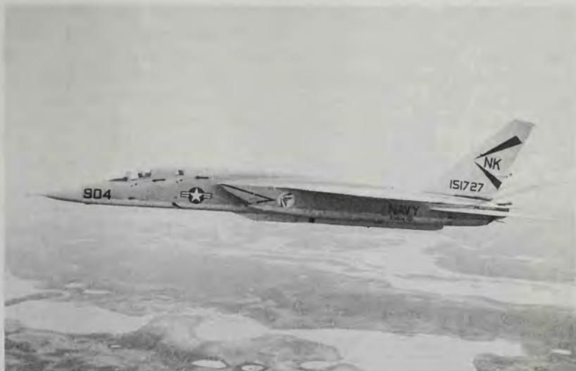
An RA-5C Vigilante from Reconnaissance Heavy Attack Squadron (RVAH) 12 shows off the aircraft's sleek lines. Note the sensor pod or "canoe" faired into the bottom of the fuselage. After the A-3 "Whale" the "Vigie" was the largest aircraft to fly regularly from carriers. (U.S. Navy)
