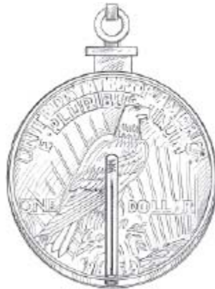
Power's silver dollar with cutaway view revealing inner pin. Phil Franke
