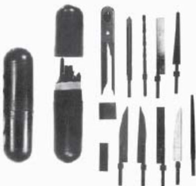
The CIA Escape and Evasion Rectal Suppository was a multipurpose tool kit packed within a smooth waterproof black plastic or aluminum shell; circa 1955 (actual size: 4” long x 1” diameter). courtesy of the authors
