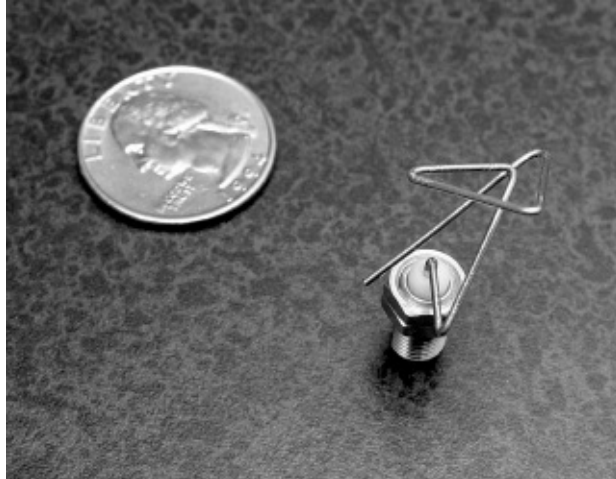
Figure 11.3 One of the small antennas designed by NASA with the help of computational selective optimization (see www.nasa.gov/centers/ames/news/releases/2004/antenna/antenna.html ).
