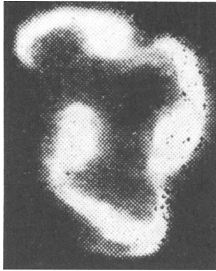
Figure 2.23. Cross-sectional view of a 2.1 mA electron beam.
