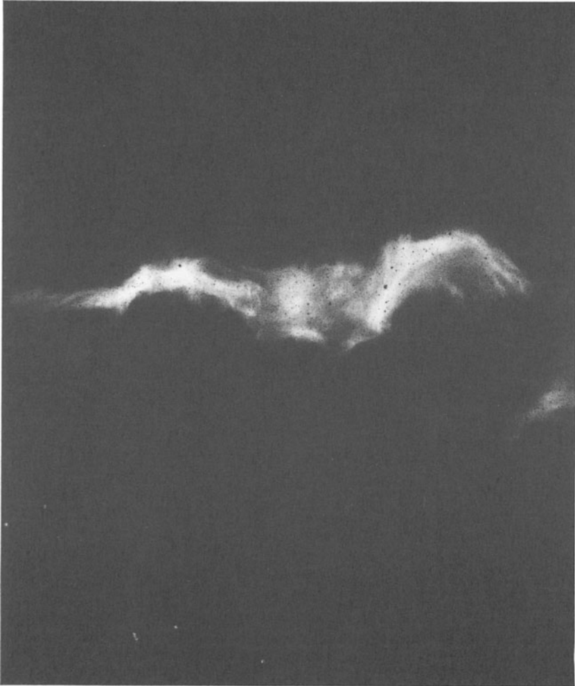
Figure 1.2. Filamentary plasma structure produced by “exploding” titanium wires within a 10 terawatt pulsed-power generator. The photograph was taken with a pin-hole X ray camera.
