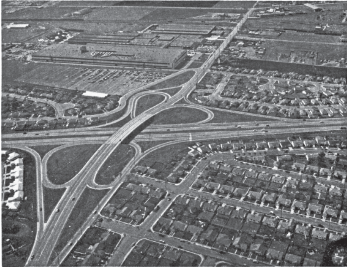
A sound street plan calls for proper integration of the four basic classes of streets. Note in this scene how the major arterial (vertical in photo) is linked with the expressway and also connects with collector streets. The latter provide access to the local streets.
