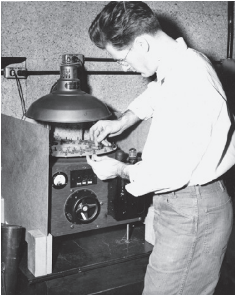
Figure 19.4 The National Bureau of Standards tests plastics for their ability to withstand weathering.
