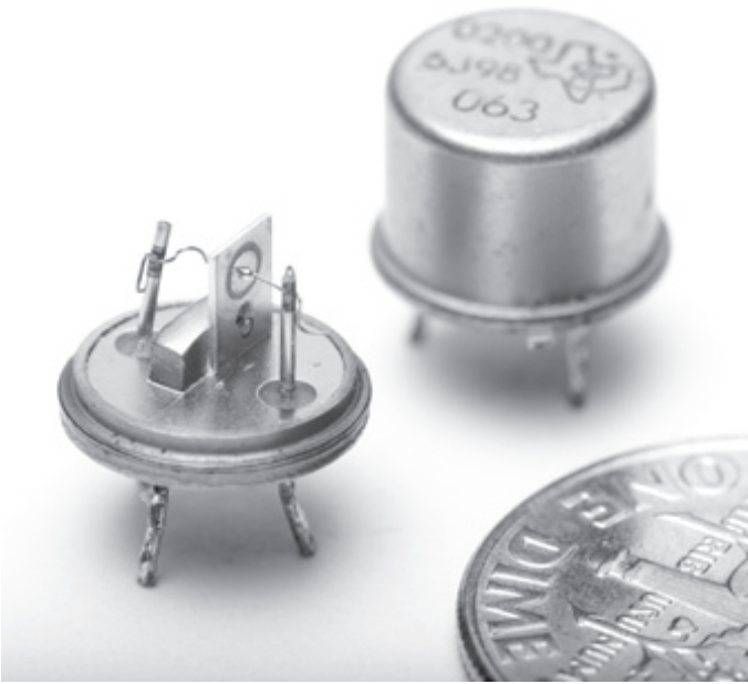
Figure 20.2 Early transistors used in the IBM 1401 (1959). In addition to the transistor's small size, the transistor did not need either a vacuum or a long warmup period.
