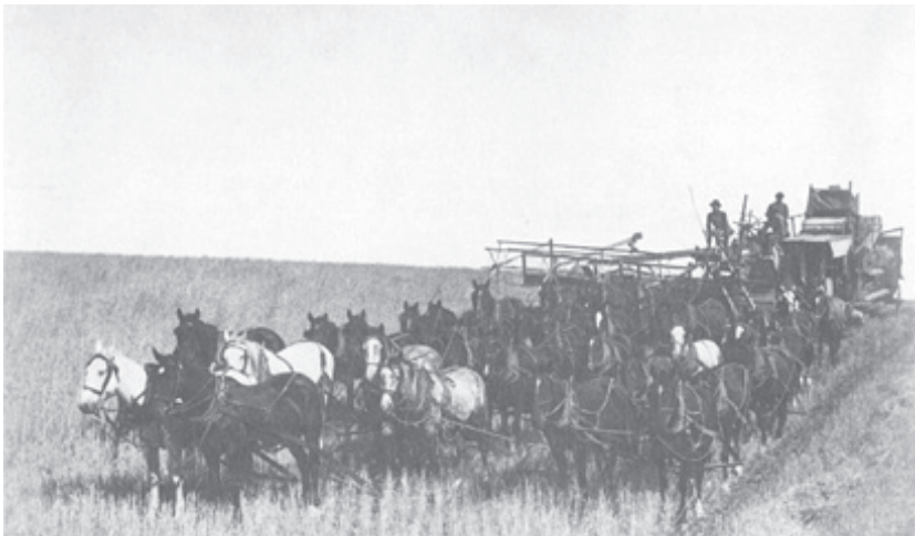
Figure 7.2 A 1903 combine (harvester and thresher). Note the number of horses, and the flat terrain, required for this 'monster' machine.
