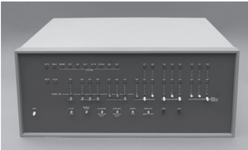
Figure 20.3 This MITS Altair 8800 was promoted to hobbyists through Popular Electronics (1975). Although primitive, this machine launched the age of the popular personal computer.
