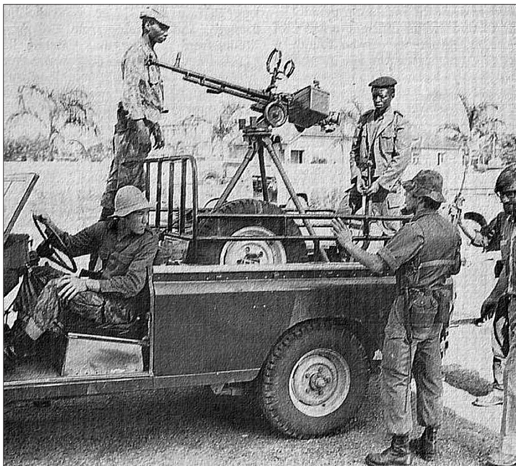
Callan gives orders to two FNLA soldiers. The gun mounted in this Land Rover is a DShK 38/46 12.7mm heavy machine gun with anti-aircraft sights. (Author's collection)
