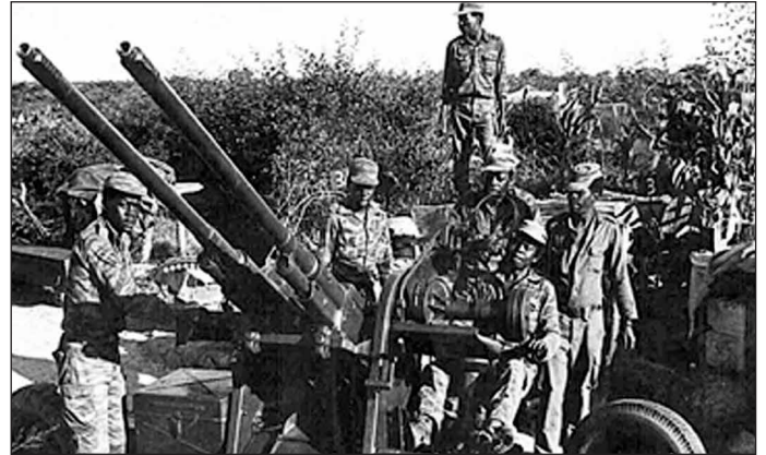
The Czech-made PLDVK vzor 53 was a towed twin-barreled 30mm anti-aircraft gun, as used on the M53/59 Praga.
