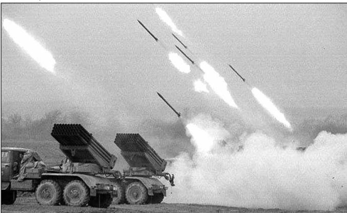
Nicknamed "Stalin's Organ", there were many variants of Soviet-made multiple rocket launchers – a formidable weapon first used by the USSR in 1939. The version deployed in Angola was the BM-21, this had a total of 40 tubes for 122mm rockets. (Author's collection)
