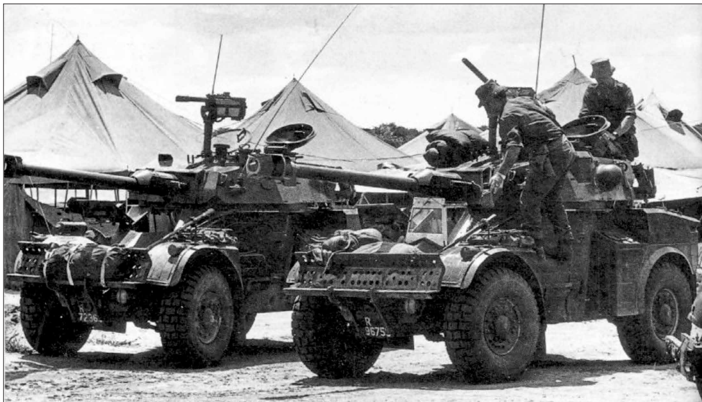
Typically, the Eland-90 was fitted with M1919 Browning 7.62mm machine guns (with 2,440 – 3,800 rounds). Its main armament was a 90mm Denel GT-2 cannon with 29 rounds, as seen here. Other variants of the Eland were armed with a 60mm breach-loading gun-mortar or a 20mm cannon.
