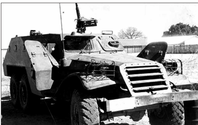
Soviet equipment used by Cuban forces included the six-wheeled BTR-152. An Armoured Personnel Carrier (APC), the BTR-152 could be equipped with a 7.62mm SG-43 Goryunov medium machine gun (1,250 rounds) or a DShK Heavy machine gun (500 rounds), but this example has a US-made Browning M1919.
