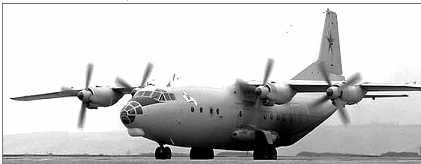
The Antonov An-12 is a four-engine turboprop transport aircraft produced between 1957-1973. The An-12 has capacity for up to 100 fully equipped paratroopers or 20,000 kg of cargo.
