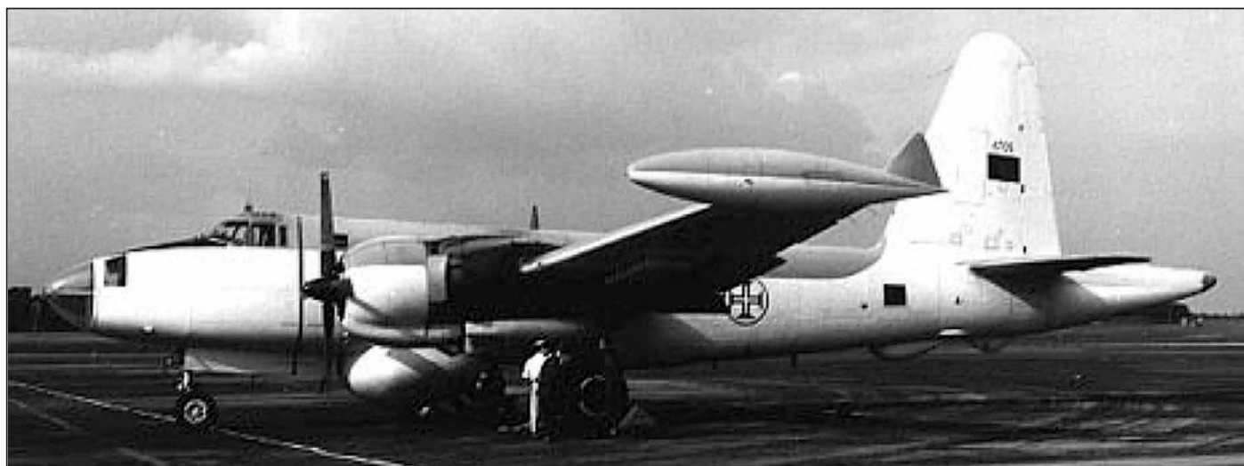
The Lockheed P2V Neptune was first introduced in 1947. A twin-engined long-range maritime patrol and anti-submarine aircraft, it was powered by two Wright R-3350-32 radial engines. In addition to its capability to carry nuclear weapons, the P2V was used by the CIA in a number of covert operations in the 1950s and used by the US Navy in Vietnam as a gunship. Later, the P2V was used by the Argentine Naval Aviation (COAN) during the Falklands War.
