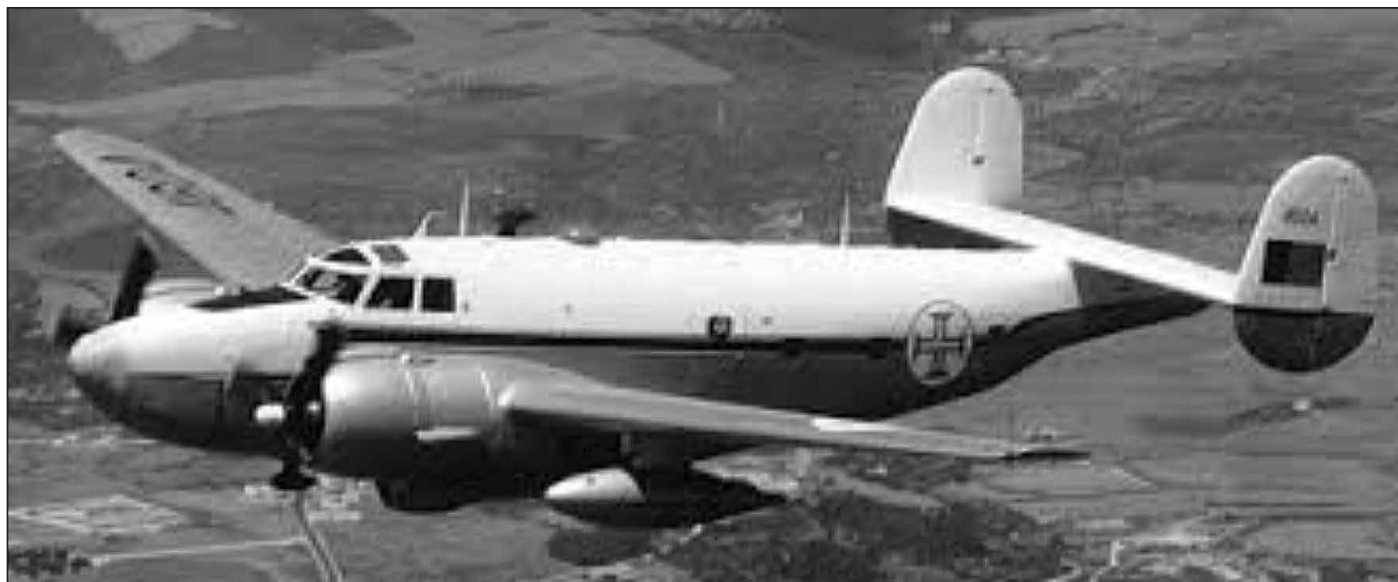
The Lockheed Ventura PV-2 Harpoon was first introduced in 1943. Used in ground attacks, the PV-2 was powered by two Pratt & Whitney R-2800-31 air-cooled radial engines. Typically, it was armed with two 0.50 cal machine guns in the upper nose decking as well as two 0.50 cal machine guns in the undernose. A further two machine guns could be placed in the dorsal turret while two others could be found in the rear ventral position. Under the wings, the PV-2 could carry eight 5-inch High Velocity Aircraft Rockets (HVARs).
