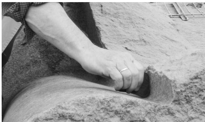
Figure 6.18. Checking the corner radius (Photograph courtesy of Dan Hamilton, 2004)
