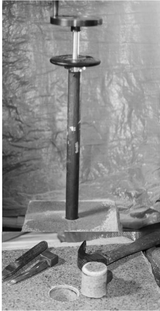
Figure 11.17. Top: Drilling rig. Bottom: Hole and core with chisel wedge and hammer.
