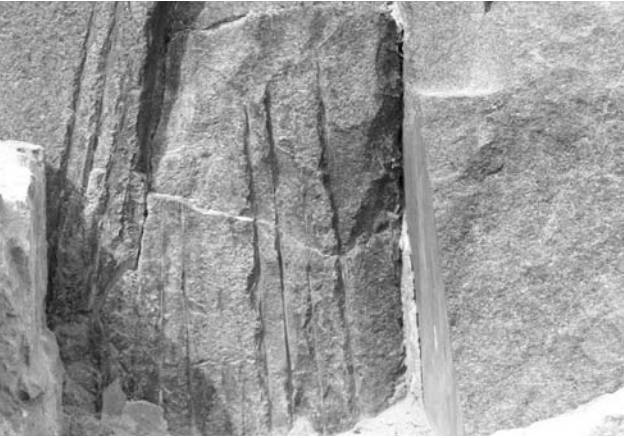
Figure 10.19. Slots sawed into basalt blocks
