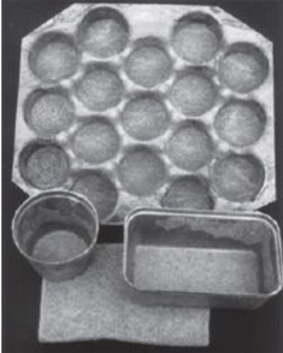
BOARDS AND CONTAINERS FROM HEMP HURDS. PHOTOGRAPH COURTESY OF INSTITUT FÜR ANGEWANDTE FORSCHUNG.
