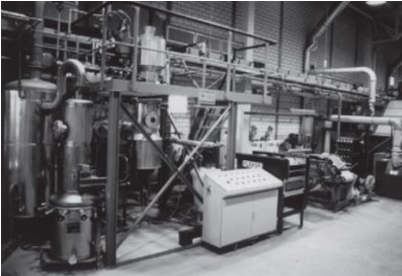
THE STEAM-EXPLOSION PROCESS: THE MARRIAGE OF HIGH-TECH SCIENCE AND AN ANCIENT PLANT . PHOTOGRAPH COURTESY OF INSTITUT FÜR ANGEWANDTE FORSCHUNG .
