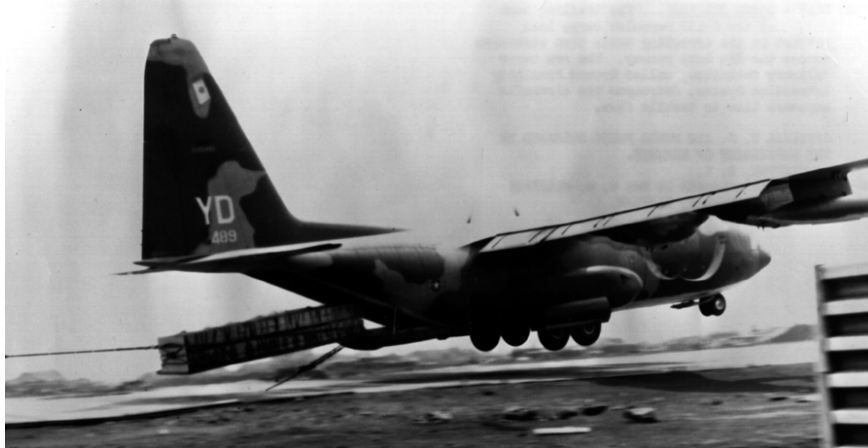
A load of cargo is pulled from an Air Force C-130 at Khe Sanh by a cable attached to the load that has snagged the runway's arrestor cable.
